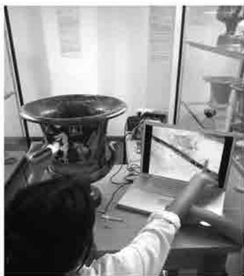
5 | Video-microscopy examination of the state of conservation of the krater.
