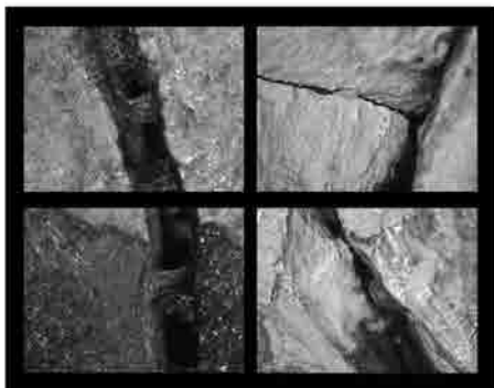
8 | Micrographs of the detachments in the krater.
